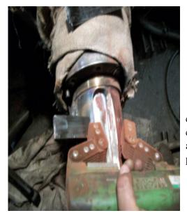
Upon further inspection by crack detection methods, Metal Surgery found that the Keyways were cracked. Metal Surgery then proceeded to excavate the cracks and prepare the shaft for welding cracked keyways and shaft complete. Then the shaft was welded by procedure.
