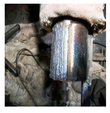
After the shaft was welded, postheat treatment and slow cooled, Metal Surgery then machined the shaft and keyways back to specifications. This shaft was machined without rotation.
