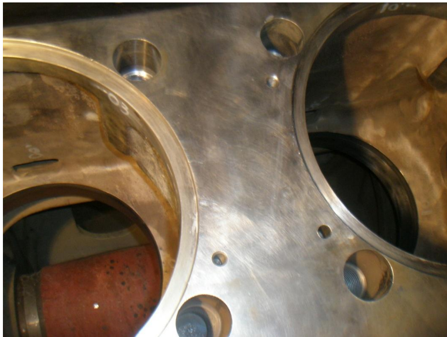
Machined and hand finished distortion .002 maximum on fire deck. All bores and bore alignment perfect. (It was another success!)
