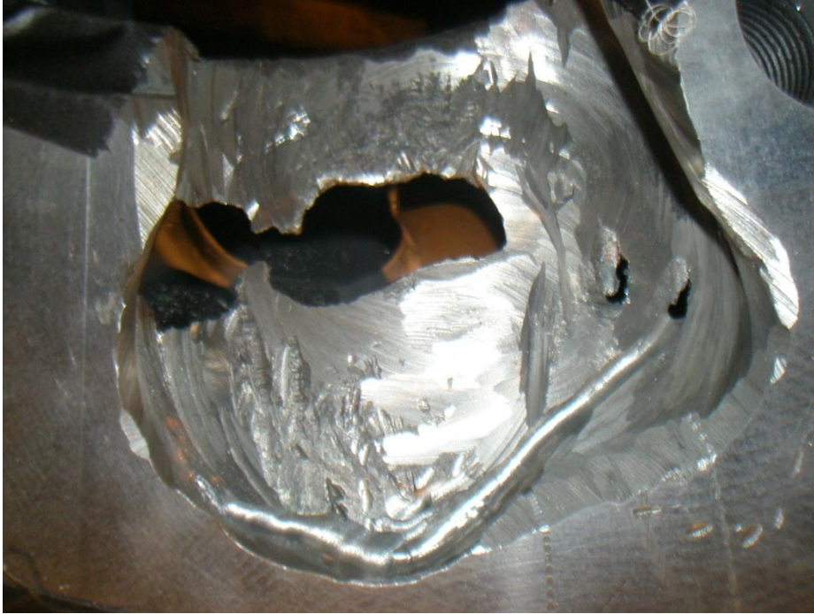
Part of the core broke out leaving a large sand inclusion approximately 8" square by 2 1/4" deep.
