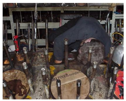
Due to the location of the crack, we had to use mirrors through the whole job. The crack was approximately 14" long. We went through over 30 large mirriors. Everytime weld or a stream of grinding sparks hit the mirror it shattered. Note the pile of mirrors in the bottom.
