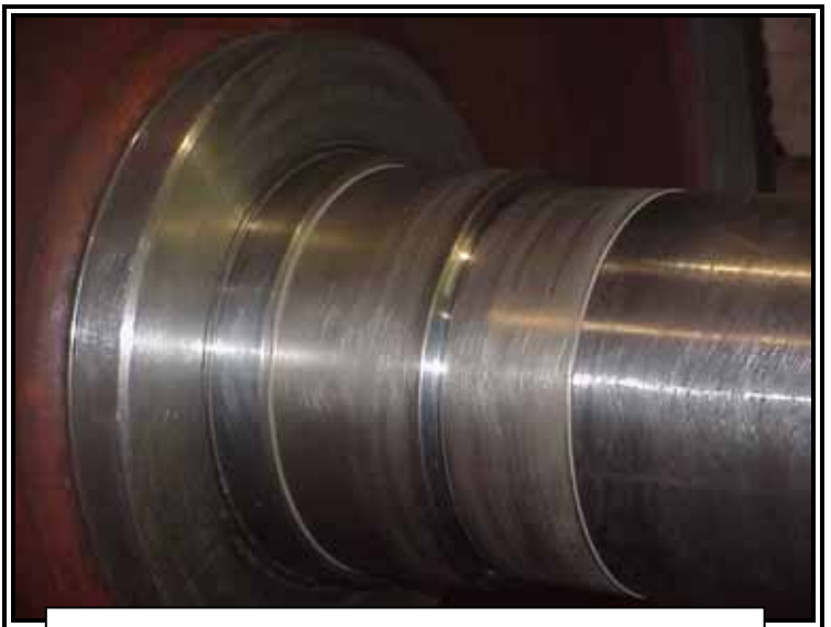
Plating repair is inspected & completed to Mfg. specifications.
