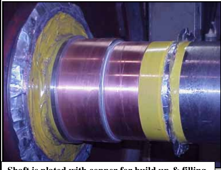
Shaft is plated with copper for build up & filling gouges from bearing failure. Also prepared for nickel plating
